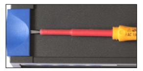
After that the upper half of the housing has to be removed. The housing is only snap-in mounted. The snap-in pins can be unlocked using a round item (approx. 5mm diameter). In the next photo a screwdriver has been used:
